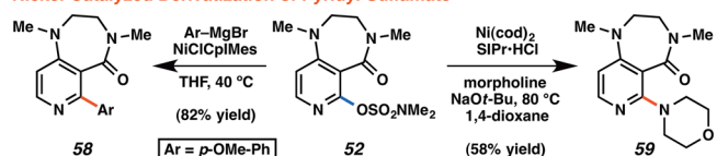
Figure 11. Functionalization of adducts 55 and 52 using transition-metal-catalyzed cross-couplings.
